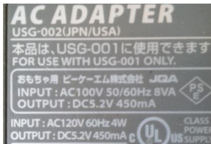
DS charger – calculate input and output separately
