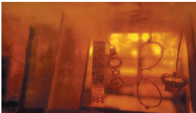
Figure 15.8 A less expensive metal can be silver-plated to produce an attractive and corrosion-resistant surface. The object to be plated is connected to a circuit as the cathode. It is suspended in a solution containing silver cyanide. The silver ions are attracted to the cathode, where they combine with electrons and become solid silver atoms that remain permanently attached to the surface of the cathode.
